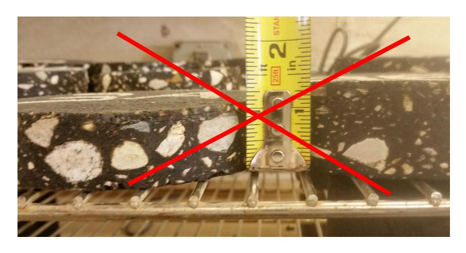
Thin lift overlays require finer mixture types!!
