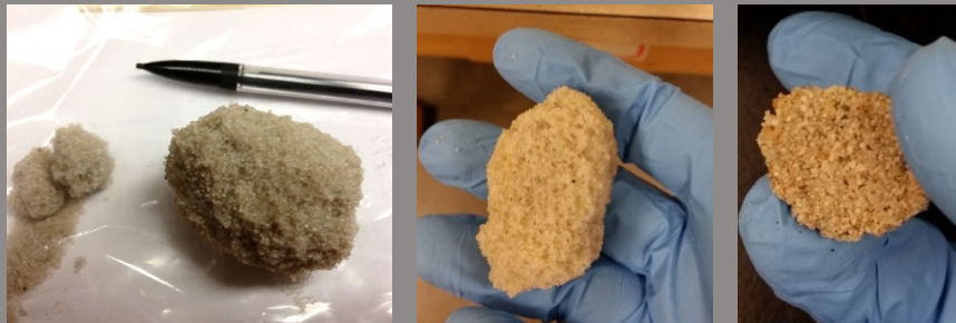
Cyclic Simple Shear Testing, Saturated Biocemented Soil
